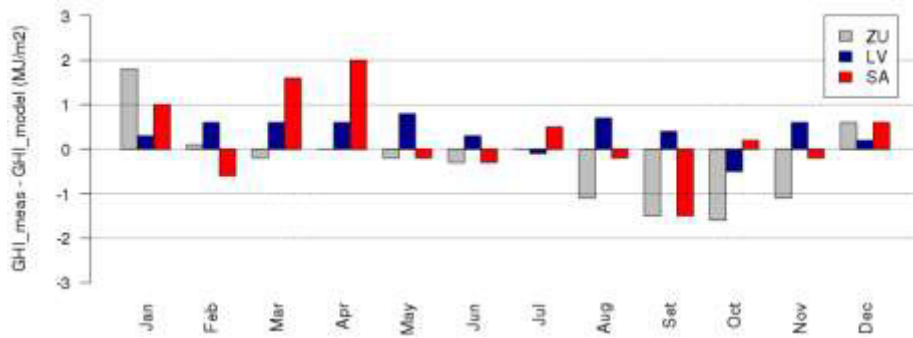
Fig. 5: Absolute deviations in \text{MJ/m}^2 between ground measurements and modeled values for daily global irradiation on a horizontal plane defined as \text{GHI (measured)} - \text{GHI (modeled)} .
