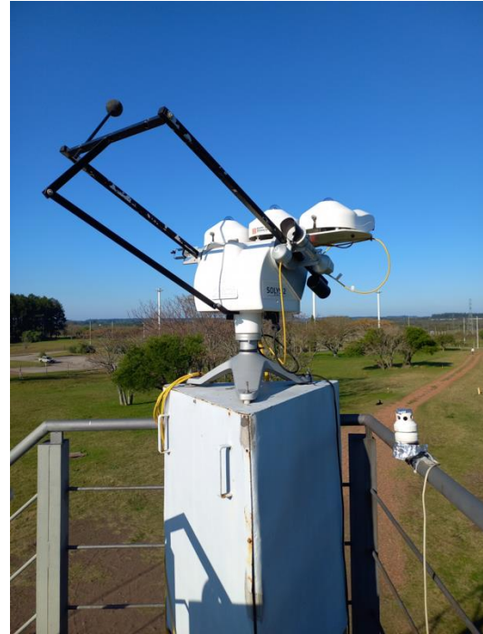
Fig. 1b: SOLYS2 system with G_d and G_b sensors.
