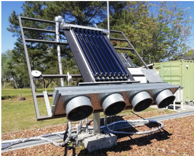
Figure 1: Assembly of the collector ETC-HP-1 on the solar tracker of the test bench.
