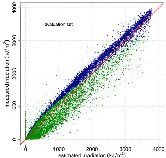
Figure 4: Scatter plot of ground data vs. satellite estimates from the JPT model (our implementation) for the EVA set on an hourly basis. Cloudy hours ( $k_T \leq 0.65$ ) are shown in green and mostly clear hours ( $k_T > 0.65$ ) are shown in blue. The measured value is used to calculate  $k_T$ . A diagonal red line has been drawn to indicate the perfect agreement case.
