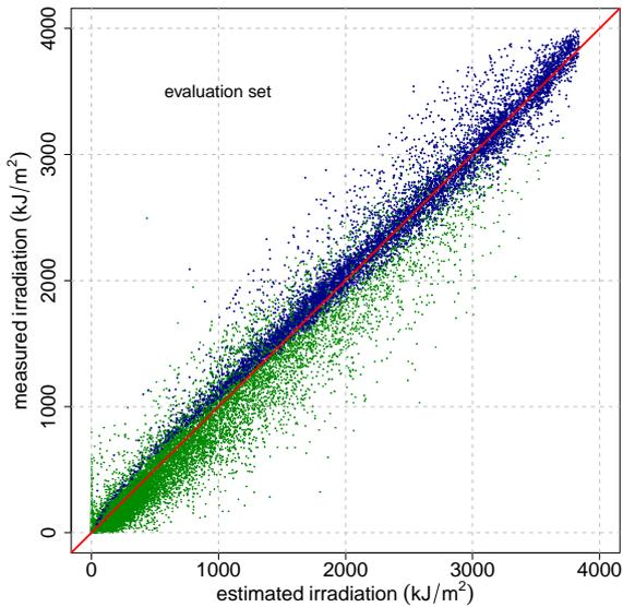
Figure 5: Scatter plot for hourly ground data vs. hourly estimates from the BD-JPT model for the four EVA sites. Green dots indicate cloudy hours, while blue dots correspond to mostly clear hours. The separation criteria is the same used in Fig. 4. The diagonal red line indicates the perfect agreement case.
