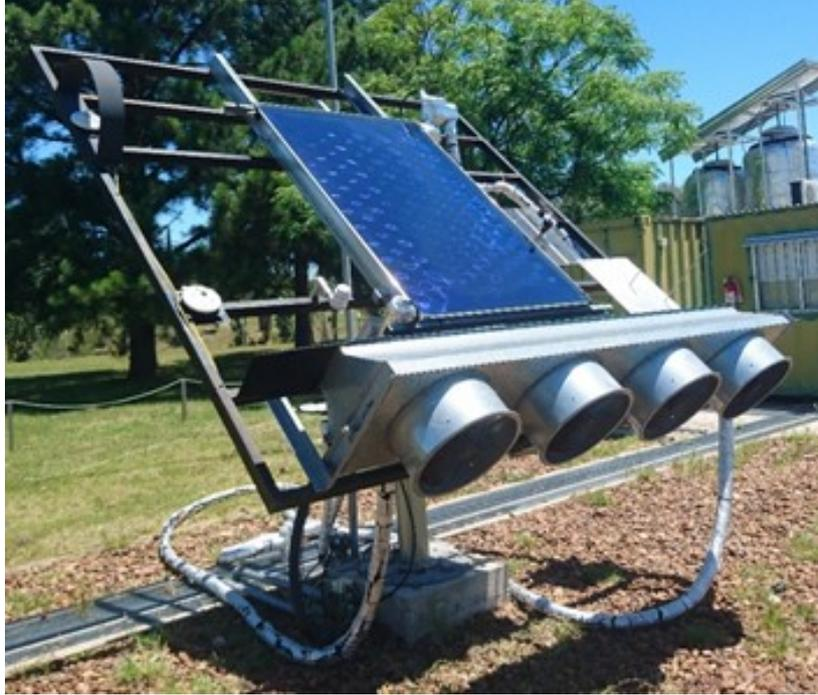
Figure 1: Assembly of the collector on the solar tracker of the test bank.
