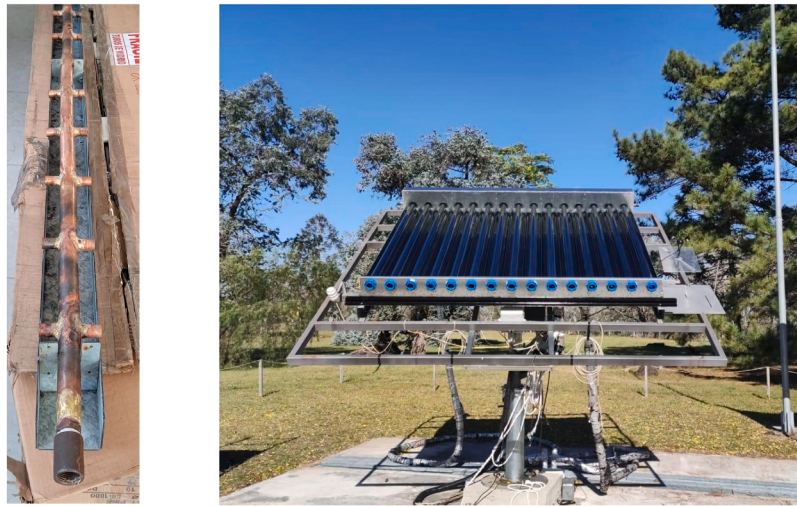
Fig. 4. Left: fabricated manifold for the first collector prototype. Right: First collector prototype mounted in the BECS.
