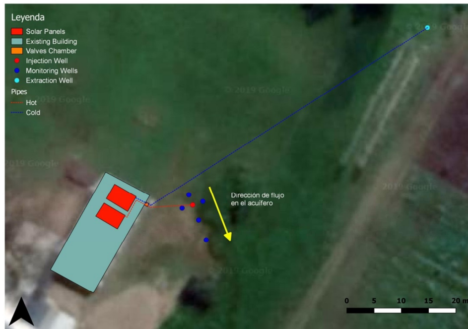
Fig. 6. Installation overview and component scheme
