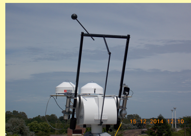
Fig. 1: Solys 2 tracker with sensing instruments
