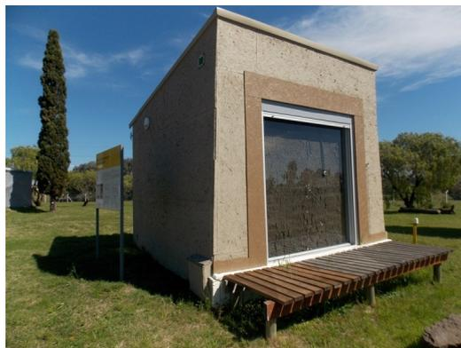
Fig. 1: Experimental setup. External compound with adobe wall oriented north, window and roll shutter.
