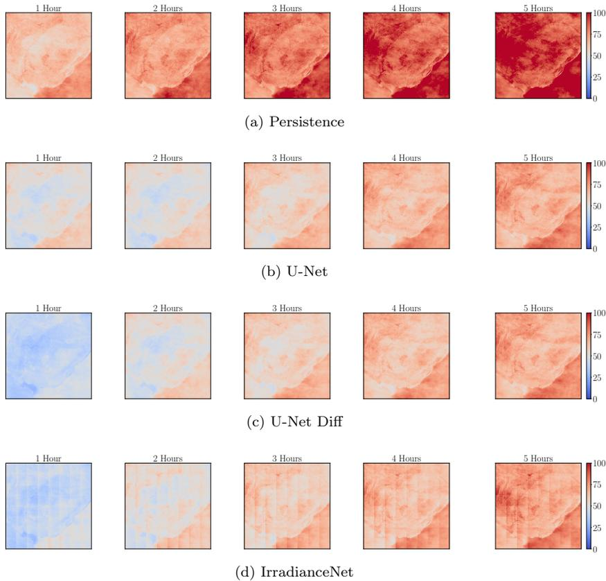
Figure 5.10: Mean relative root squared error per pixel for all five time horizons. On the REGION3 test dataset.
