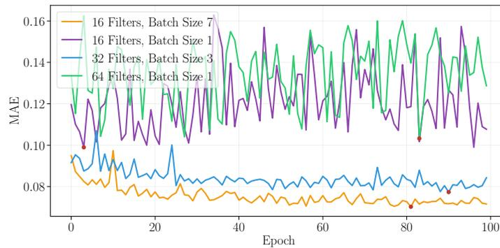
Figure 4.7: Validation learning curves for the U-Net with different initial filters and batch size, over the REGION3 validation dataset. The red dots mark in which epoch the model reached the minimum error.
