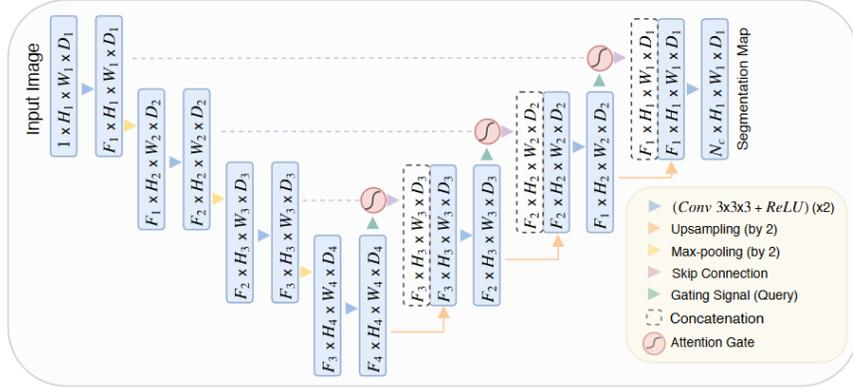
Figure B.1: A block diagram of the proposed Attention U-Net segmentation model. Attention gates (AGs) filter the features propagated through the skip connections. Schematic of the AGs is shown in Figure B.2. Feature selectivity in AGs is achieved by use of contextual information (gating) extracted in coarser scales. Figure reproduced from [46].
