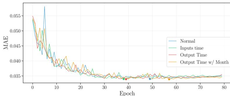
Figure 4.17: Validation learning curves using MAE in the MVD dataset adding the time of images as an input, with a prediction horizon of 10 minutes
