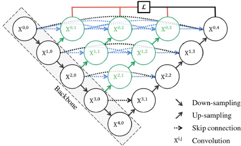
Figure B.4: UNet++ architecture consists of an encoder and decoder that are connected through a series of nested dense convolutional blocks. Figure taken from UNet++ [45].
