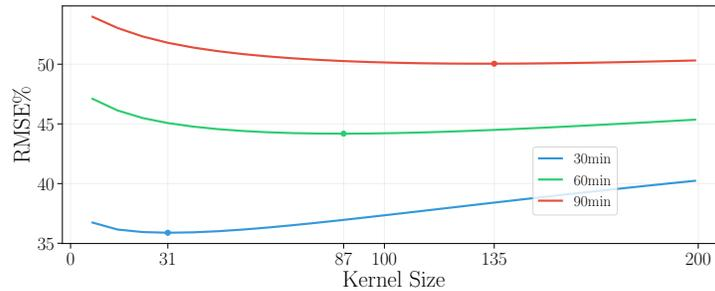
Figure 4.2: Kernel size optimization of blur applied to CMV for MVD. Calculated as the average in the MVD validation dataset, for 30, 60, and 90 minutes prediction horizons.
