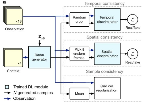
Figure 3.3: DGMR architecture. Figure taken from "Skilful precipitation nowcasting using deep generative models of radar" [22].
