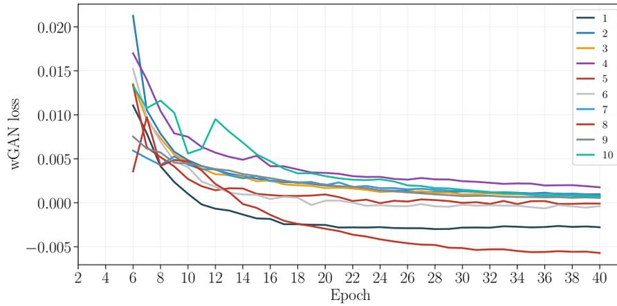
Figure C.11: Training learning curves using wGAN loss for every epoch for the 10 best models, using U-Nets with 16 filters trained for 40 epochs to predict 30 minutes into the future.
