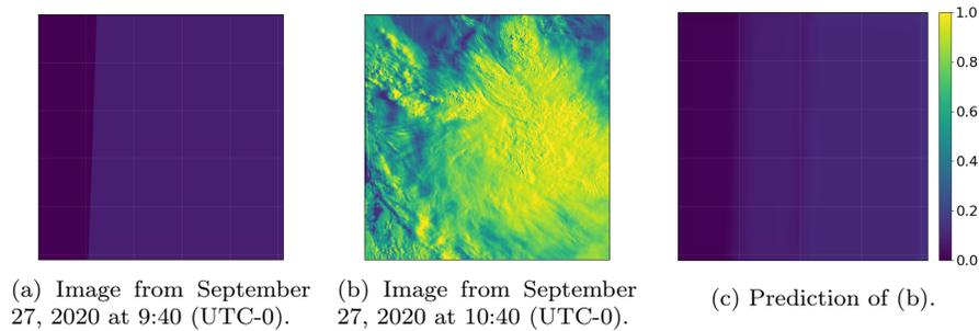
Figure 4.9: Prediction made with the U-Net (16 filters) over REGION3 during sunrise. Image (a) is the last input, and image (b) is the ground truth one hour after (a). Image (c) is the prediction of (b).
