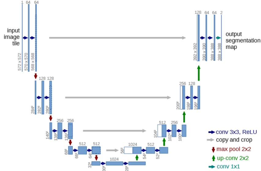
Figure 3.6: U-Net Original Architecture. Figure taken from U-net: Convolutional networks for biomedical image segmentation [34].
