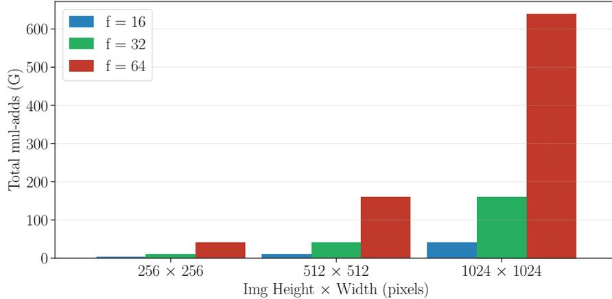
Figure 3.9: Number of operations done in one forward pass according to the initial filters ( $f$ ) and image size.
