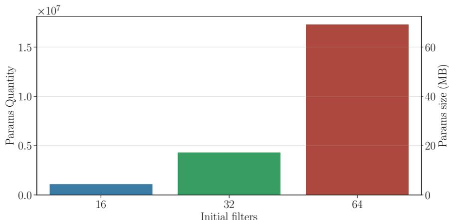
Figure 3.7: On the left y-axis it is marked the quantity of trainable paramas for different number of initial filters. The right y-axis shows the size it takes to allocate those paramas.
