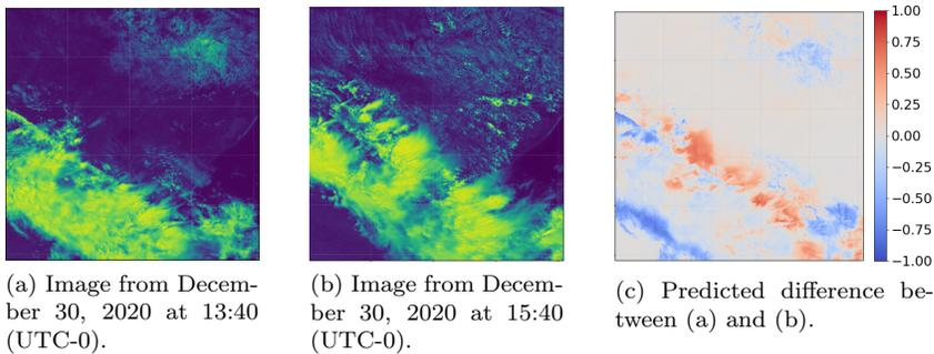
Figure 4.15: Example of the output of the U-Net Diff when predicting at a 2 hours prediction horizon.
