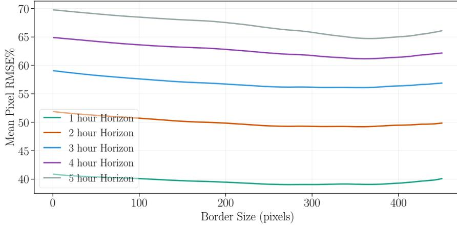
Figure 5.11: Optimal cropping for the test dataset for RMSE%. Done using U-Net Diff.
