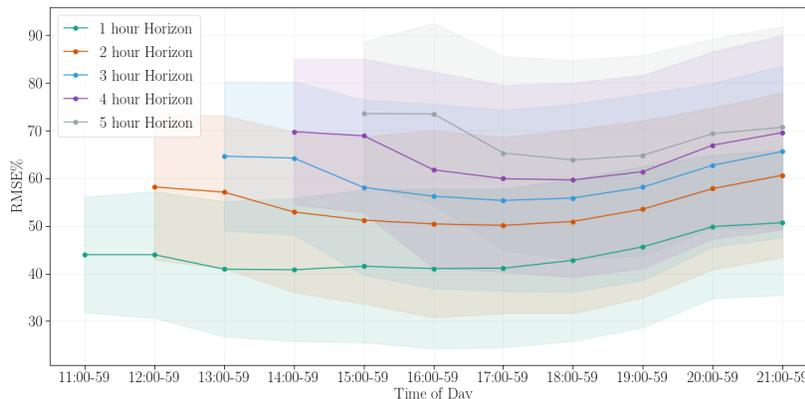
Figure 5.14: Mean RMSE% value with the standard deviation for all images in hourly non-overlapping time frames, for all five prediction horizons, using the U-Net Diff for each hour of the day covered in the dataset. Timezone: UTC-0.
