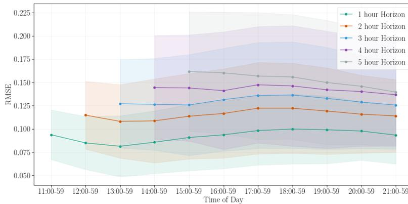
Figure 5.13: Mean RMSE value with the standard deviation for all images in hourly non-overlapping time frames, for all five prediction horizons, using the U-Net Diff for each hour of the day covered in the dataset. Timezone: UTC-0.
