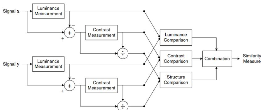
Figure 3.1: SSIM measurement system diagram. Figure extracted from [31].
