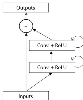
Figure B.6: Recurrent Residual Convolutional Unit (RRCU) diagram. Figure taken from R2U-Net's paper [47].
