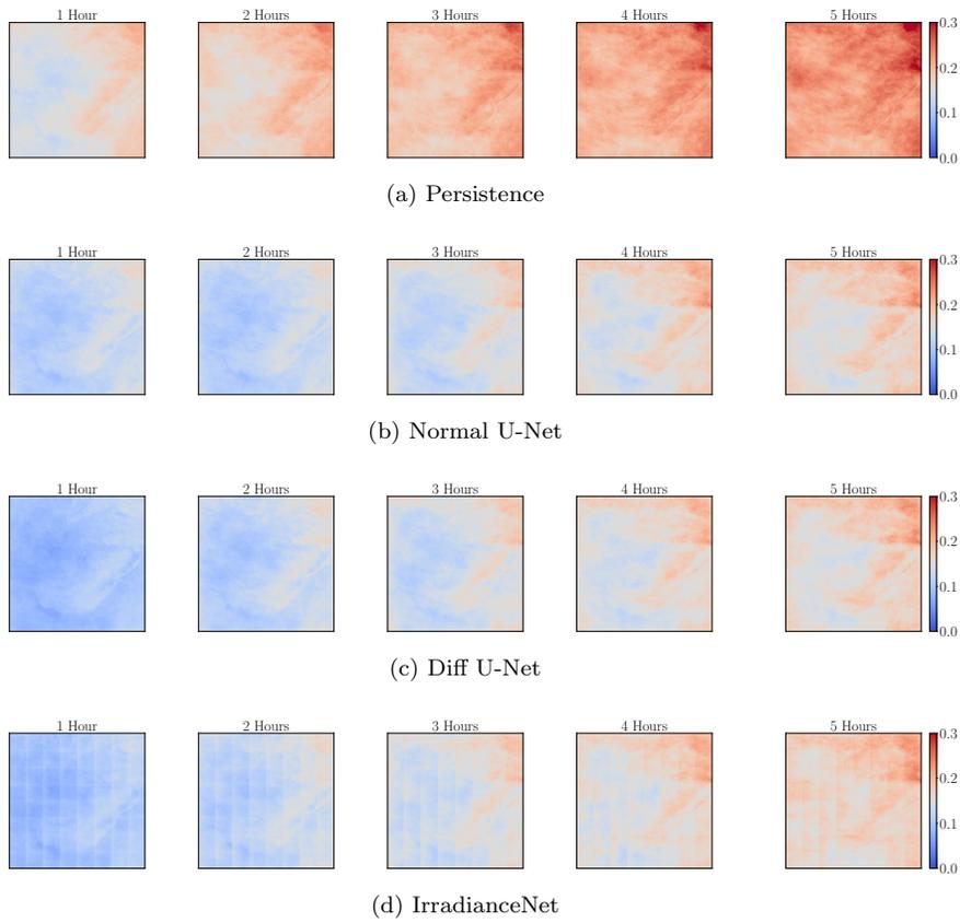
Figure 5.6: Mean root squared error per pixel for all five time horizons. On the REGION3 test dataset.
