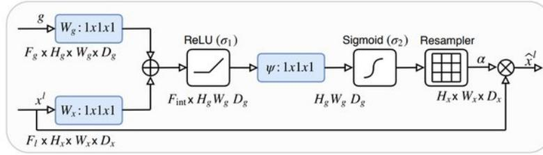
Figure B.2: Schematic of the proposed additive attention gate (AG). Input features ( $x^l$ ) are scaled with attention coefficients ( $\alpha$ ) computed in AG. Spatial regions are selected by analysing both the activations and contextual information provided by the gating signal ( $g$ ) which is collected from a coarser scale. Grid resampling of attention coefficients is done using trilinear interpolation. Figure reproduced from [46].
