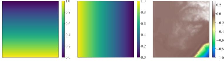
Figure 4.18: Spatial data used for training IrradianceNet GEO on the REGION3 dataset. The first two images inform from where the patch was taken (simulating the geographic coordinates), the third image is the elevation of the region with normalization.
