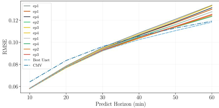
Figure 4.20: RMSE loss on validation evaluated recursive up to 1 hour on the 10 best models according to RMSE loss on validation, in their peak validation performance.
