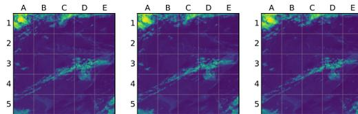
Figure D.1: Image sequence used as input for the U-Net Diff and CMV algorithm. Captured on January 13, 2020 at 12:00, 12:10, 12:20 (from left to right). Timezone UTC-0.
