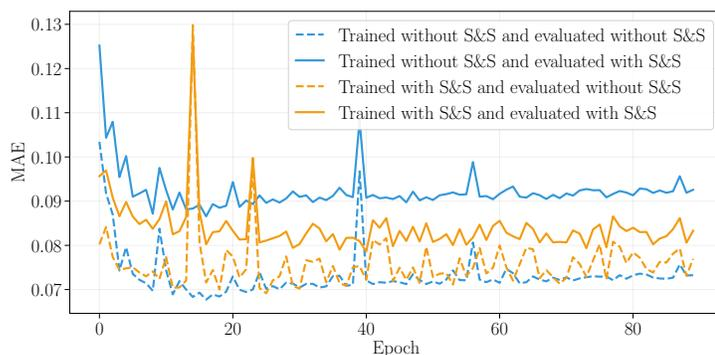
Figure 4.12: Validation curves for the U-Net trained over the URU dataset. The orange curves are trained using the dataset with S&S, the blue ones without. The solid lines are evaluated using the dataset with S&S, the dashed ones are evaluated in the dataset without.
