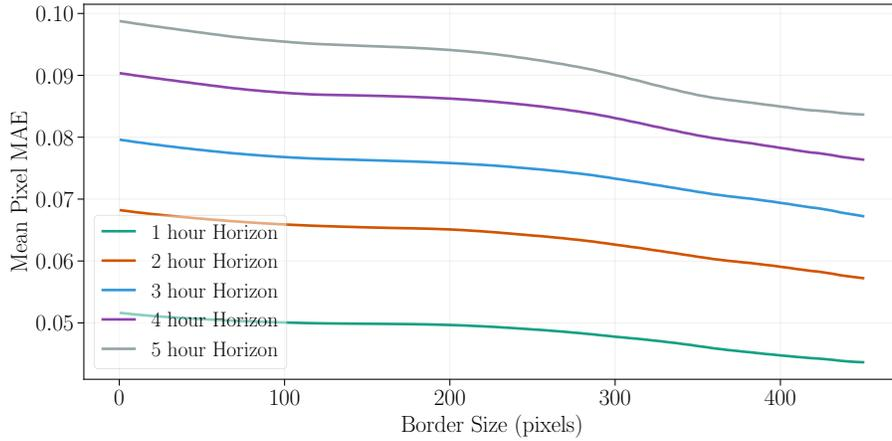
Figure 5.8: Mean error for the U-Net Diff for different windows for the 5 horizons on the REGION3 test dataset.
