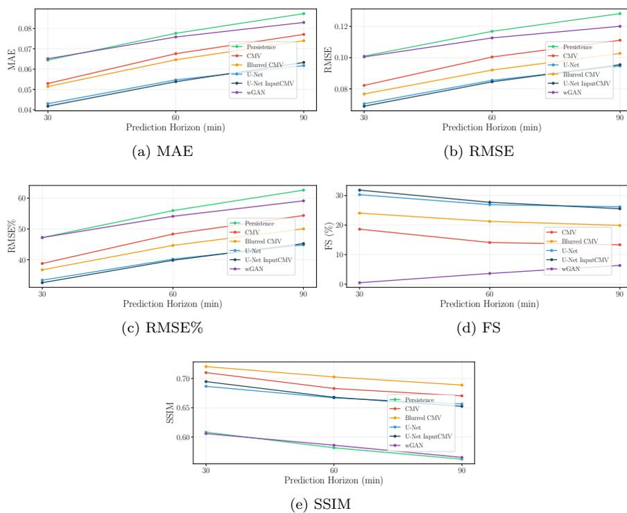
Figure 5.15: Performance comparison in MVD test dataset. The algorithms evaluated are Persistence, CMV, Blurred CMV, U-Net, U-Net InputCMV and wGAN. The metrics used to generate the figures are MAE (a), RMSE (b), RMSE% (c), FS (d), and SSIM (e).
