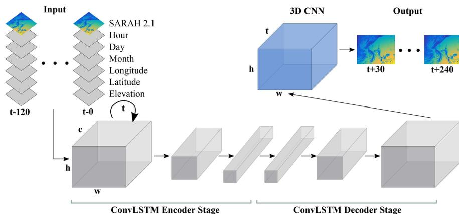
Figure 3.10: IrradianceNet Architecture. Figure taken from IrradianceNet: Spatiotemporal deep learning model for satellite-derived solar irradiance short-term forecasting [41].
