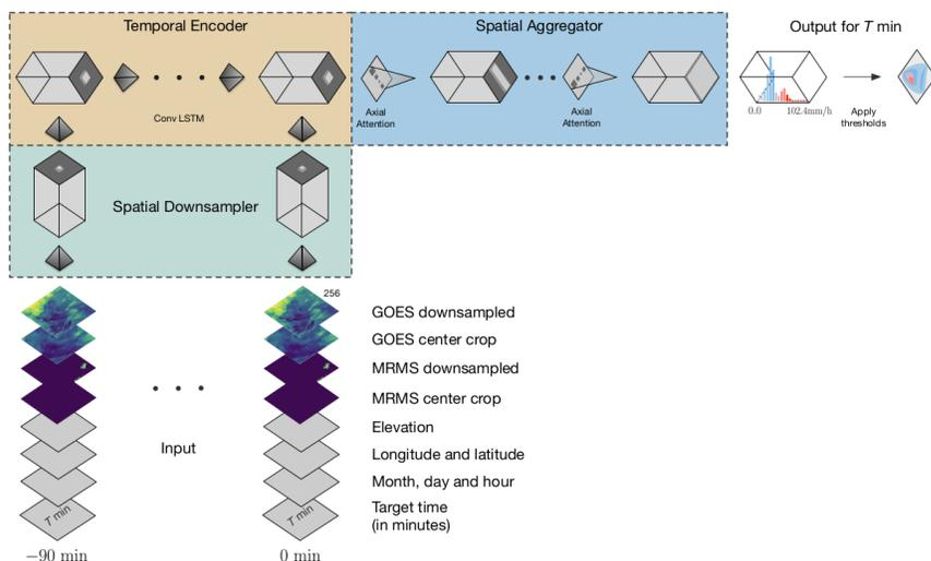
Figure 3.4: MetNet architecture. Figure taken from "MetNet: A Neural Weather Model for Precipitation Forecasting" [13].
