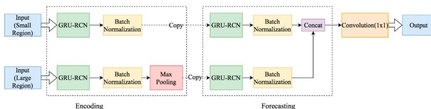
Figure 3.2: Multi-GRU-RCN architecture. Figure taken from "Prediction of Short-Time Cloud Motion Using a Deep-Learning Model" [35].
