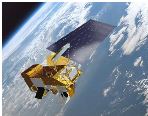
Figure 2.14: Aqua Satellite from NASA https://oceancolor.gsfc.nasa.gov/about/missions/aqua/ , which carries on board the MODIS Spectroradiometer.
