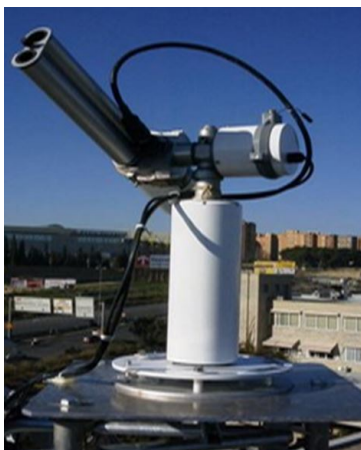
Figure 2.13: CIMEL sun photometer (extracted from: https://aeronet.gsfc.nasa.gov/new_web/photo_db_v5/Burjassot.html )
